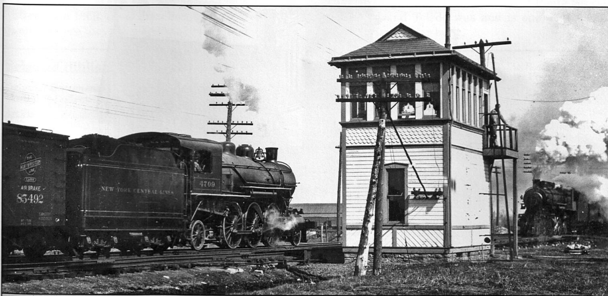
Here is a rare action shot of one of the 35 J-41 2-6-2 Prairie-type locomotives built by Alco-Brooks between October 1904 and February 1906. The 4708 is heading east past Bay Junction Tower, where the LE&W crossed the main line just south of Sandusky. Photo by Ernst Niebergall. Charles E. Frohman Collection/Hayes Presidential Center.
