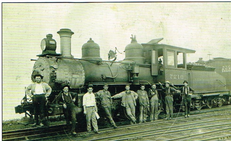
The Big Four's presence in Sandusky is represented here by CCC&St. L 7216, an 0-6-0 switch engine constructed for the Cincinnati, Sandusky and Cleveland Railroad by the Rome Locomotive Works in 1889. Sandusky Public Library.
