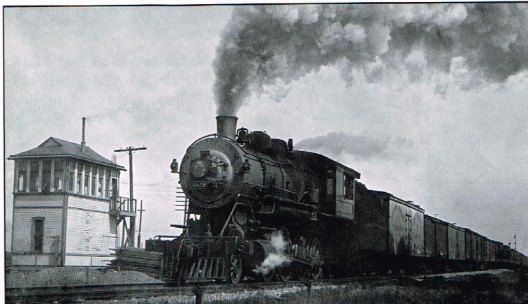
Lake Erie & Western 2-8-0 5329, a Class G-44 locomotive built by Brooks in 1904, bats No. 66, a daily LE&W westbound hotshot, past Bay Tower. A vintage string of truss-rodded reefers and boxcars follows. The fireman ponders who this man with a camera might be. Photo by Ernst Niebergall. Charles E. Frohman Collection/Hayes Presidential Center.
